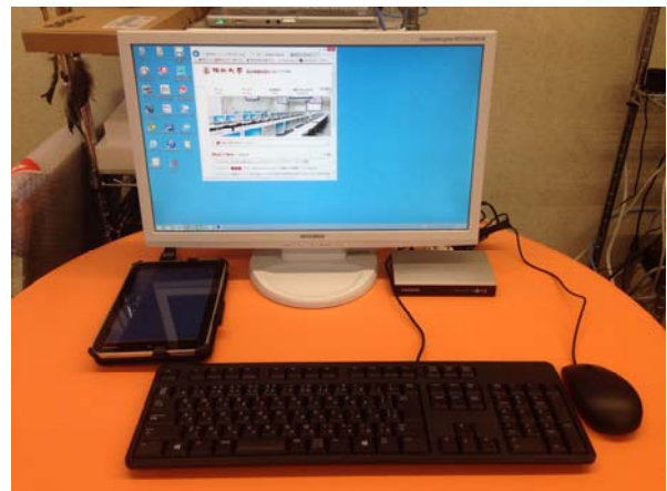
Fig. 4 The docking station and Tablet PC are connected by a single USB cable
